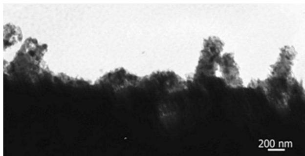
**FIGURE 6:** TEM image of a polyaniline-nanodiamond film composite
