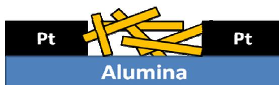
Fig. 2 Schematic view of the  $\text{TiO}_2$ /CNFs sensing layer deposited on the patterned alumina substrate.
