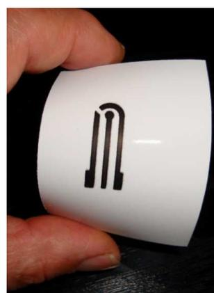
Fig.2 Inkjet printing of MWCNT/AgNPs-PMA thin films as electrodes on flexible substrate.
